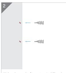
Using the marks from step 1, drill and install appropriate screw anchors for the application. (not included)
