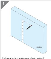
Using a tape measure and wax pencil, mark the intended location on the glass. If applicable, refer to ADA installation requirements.
