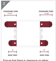
Ensure that there is clearance on either side of sign to allow tabs to slide unobstructed. (4-1/2" for Standard Tabs, 3" for Mini Tabs).
