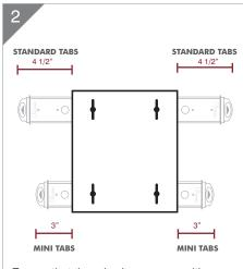
Ensure that there is clearance on either side of template to allow tabs to slide unobstructed. (4-1/2" for Standard Tabs, 3" for Mini Tabs).
