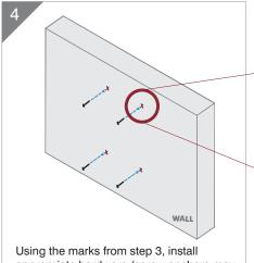
Using the marks from step 3, install appropriate hardware (screw anchors may be required). Screws must be no larger than #6 and are not provided.
