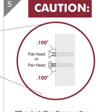
When installing the mounting screws, ensure to leave .100" of clearance to allow the sign to slide firmly into place.
