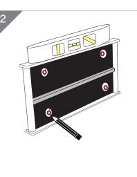
Use a level to place the system to its intended location and mark the mounting hole locations. Refer to ADA requirements if applicable.
