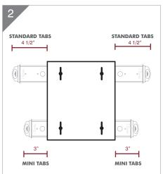
Ensure that there is clearance on either side of template to allow tabs to slide unobstructed. (4-1/2" for Standard Tabs, 3" for Mini Tabs).
