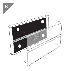
Reinsert paper insert (if present) and non-glare lens. Ensure that the non-glare side faces out.
