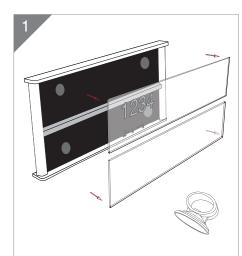
Using provided suction cup, gently remove the non-glare lens and paper insert (if present).
