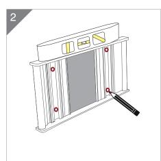
Use a level to place the system to its intended location and mark the mounting hole locations. Refer to ADA requirements if applicable.
