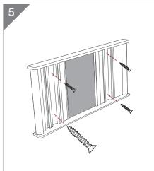
Align mounting holes to the wall anchors and permanently secure system to wall using appropriate hardware. (not included)
