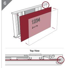
Reinsert black support panel, ensuring that it sits in the furthest position slot. Then reinsert paper insert (if present) and nonglare lens. Ensure non-glare side faces out.
