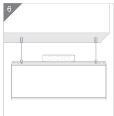
Raise the sign into place and using the provided 2mm allen wrench (3mm for HID Systems), tighten the set screw until closed. Make certain that your sign is level.
