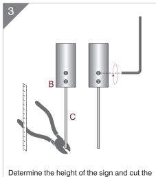
Determine the height of the sign and cut the provided cables (C) to identical lengths. Secure the cables to the ceiling barrels (B) using the provided 2mm allen wrench.
