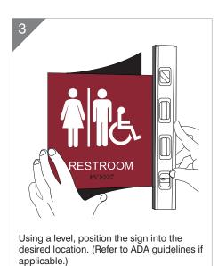
temporarily fasten system to wall for
